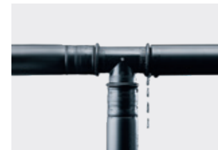
Defined leak paths make unpressed fittings immediately visible in the pressure test.
