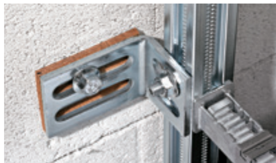
↑ The Geberit GIS mounting brackets with sound insulation bases made of cork ensure that the support system is securely anchored and reliably sound decoupled.
