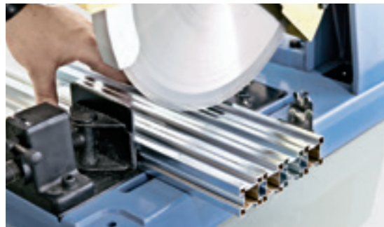
↑ Up to four Geberit GIS profiles can be cut to length at the same time with the chop saw.
