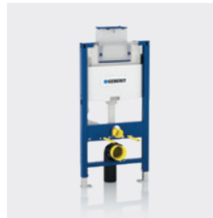
↑ Geberit Duofix element for wall-hung WC, 82 cm, with Omega concealed cistern.
